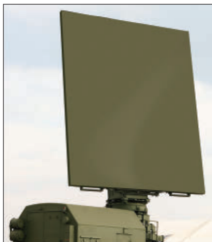
▲ Fig. 1 The active phased array architecture enables the beam to be electronically steered and multiple radars to be combined in a single system.
